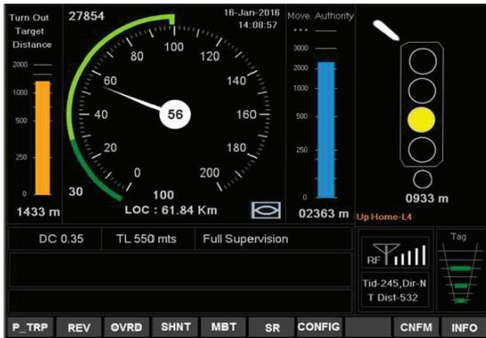
Figure 2: Loco Pilot Machine Interface
