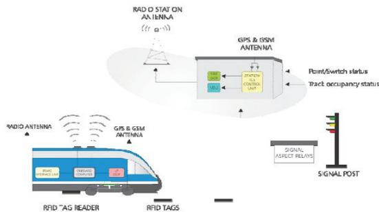
Figure 1: Indigenous Train Protection System of RDSO
