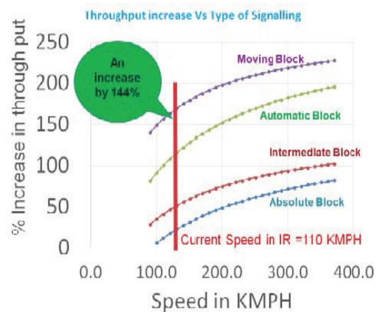
Figure 3: % Increase in Through-put with advanced Signalling Systems
