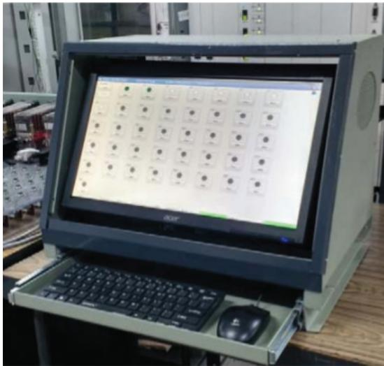
Figure 2: VDU based SM's Reset Panel
