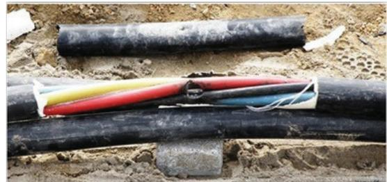
Figure 2: Electrical cables damaged when laid without Cable Channel
