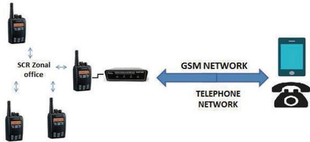
Figure 3: UHF Walkie-Talkie working through GSM network
