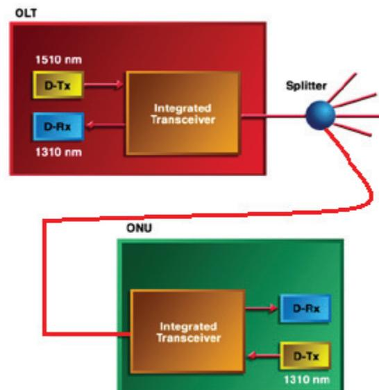
Figure 5: 2-Wavelength Ethernet PON
