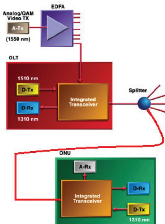
Figure 6: 3-Wavelength Ethernet PON
